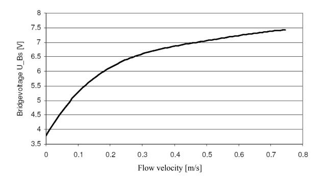
Typical signal – curve between 0 .... 0.8 m/s
